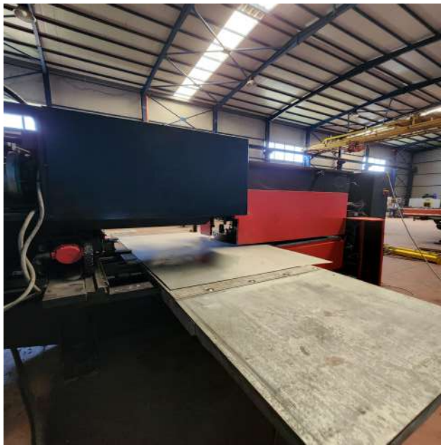
Punching machine The machine that opens holes of different sizes and coordinated shapes is the CNC, Amada
