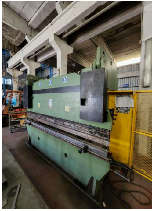
CoraMut bending machine 100 Tons For the return of sheet metal, thickness from 0.4 to 3 mm, with a length of 3 m
