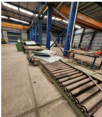
The spencer, which carries out the flattening / straightening of the sheet metal of the trays with a width of 1250 mm and in the required length, by Spencer from 0.5 mm to 2.5 -3 mm
