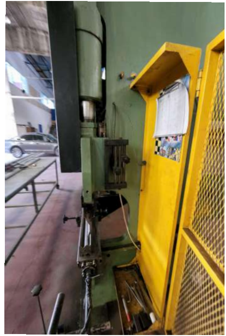
CoraMut bending machine 100 Tons For the return of sheet metal, thickness from 0.4 to 3 mm, with a length of 3 m
