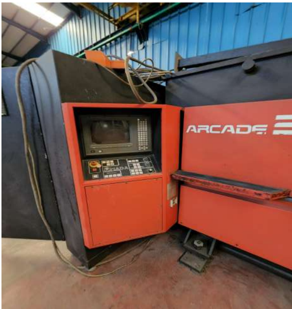
Punching machine The machine that opens holes of different sizes and coordinated shapes is the CNC, Amada
