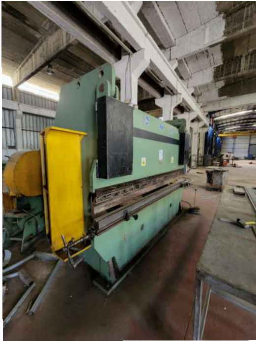
CoraMut bending machine 100 Tons For the return of sheet metal, thickness from 0.4 to 3 mm, with a length of 3 m
