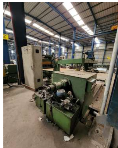
The spencer, which carries out the flattening / straightening of the sheet metal of the trays with a width of 1250 mm and in the required length, by Spencer from 0.5 mm to 2.5 -3 mm
